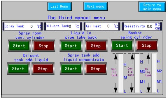
•Cleaning (spray) room vent cylinder: Click Start or Stop to start or stop air vent cylinder on top of spray (cleaning) room.
