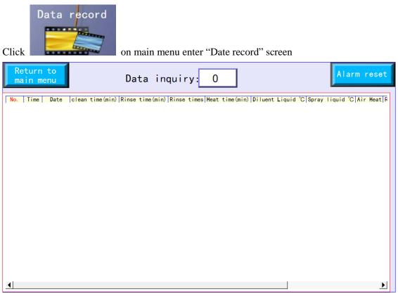
Data record is used to record setting parameters such as (cleaning) time,(diluent liquid) temperatures...for the convenience of data inquiry.
